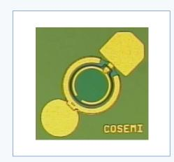
Cosemi's SPD2004 is a short-wavelength, mesastructured, GaAs-based PIN photodiode offering high responsivity, low dark current and low capacitance for high bandwidth, high performance optical receiver designs.
